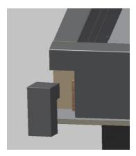
• Fast the allen screws tightly and use two further screws per angle bracket at each side.
