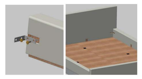
• Now fasten 2 more angle brackets per side to the side parts and the base boards.
