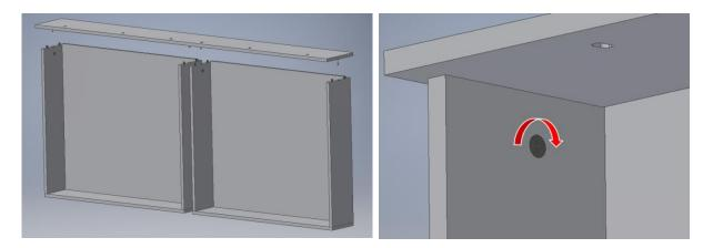
4. The upholstered front is fastened with screws as illustrated, but not too tight at this point.
