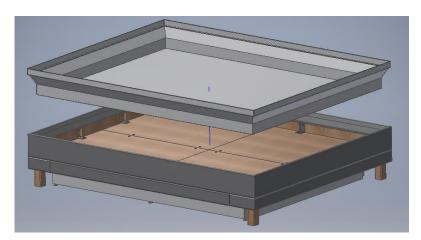
12. The heating elements are placed on each side of the bed at the head end. The cables are led through the holes in the bottom plates and in the lower part of the cover.
