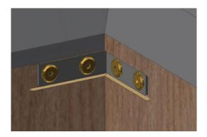
10. A bed leg is secured to each corner. A lock washer is placed between the leg and the bottom plate.
