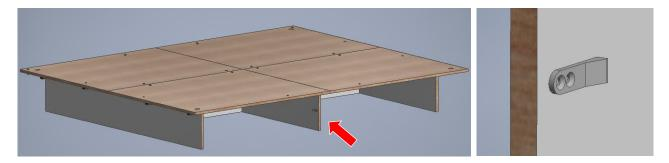
7. The long sides of the frame and the foot end are positioned with angle brackets, but not fastened too tight at this point. (**This applies for beds with an upholstered frame**.)
