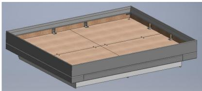
9. Angle brackets are fastened loosely at the corners. Then the screws at each corner are tightened one by one beginning with the inner screws. After this the angle brackets connecting the bed frame and the base are tightened. Two angle brackets are fastened at each corner.
