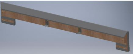
8. The bed frame is positioned on the base without fastening the screws of the angle brackets too tight.
