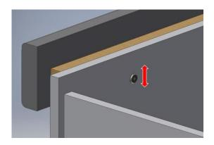
6. A steering plate for the drawers is screwed to each side of the central base section. Place them staggered to avoid the screws hitting each other.
