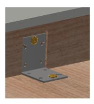
• The angle brackets are tightened loosely at the corners. Then one by one the screws at each corner are tightened firmly. It is important to begin with the inner screws. After this the angle brackets are all to be tightened firmly.
