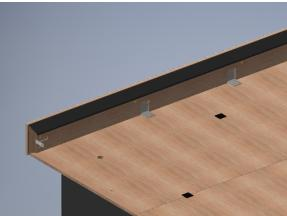
• Dowels and angle brackets are placed in the hed- and foodend frame parts. These parts are positioned on the bed and fasted to the long side parts of the frame. Finally tighten all screws firmly.
