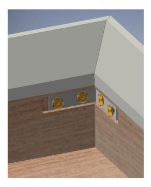
• **Wooden frame:** the frame parts are assembled with angle brackets that are to be tightend firmly. Then screw the angle brackets to the bottom plates, position the frame parts and screw them to the bottom plates, but not quite 100% firm yet.
