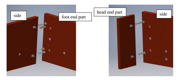
3. The suspension parts are attached to the foot end and side frames.
