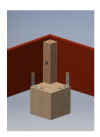
5. Bottom plates are fitted to the base.
