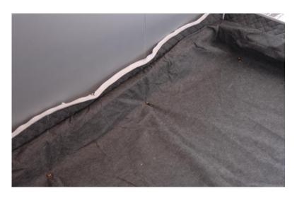
• The upper foam side parts are positioned, then the upper foam end parts. The keyholes are lowered onto the screws. Then the sides are pushed into place, and finally the screws are tightened.
