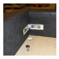
• The frame parts are secured to the bottom plates. In each frame part there are threaded bushings for 2 angle brackets, and in the side parts there is an additional treaded bushing at each end. Fasten the screws. The distance from the top of the screws to the bottom plates should be approximately 1 cm.
